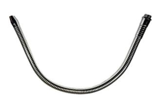
FLEXIJET<sup>®</sup> with fixed nozzle J-60-3/8, d male thread 3/8 '', chrome plated, LG 600 mm
